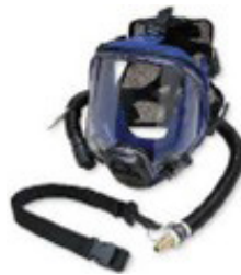
EN138: a fan-assisted fresh air hose with full-face mask providing the fresh airline hose inlet can be located well away from the work area, e.g. outside the building and upwind of any local sources of airborne contamination, such as vehicle exhaust.
